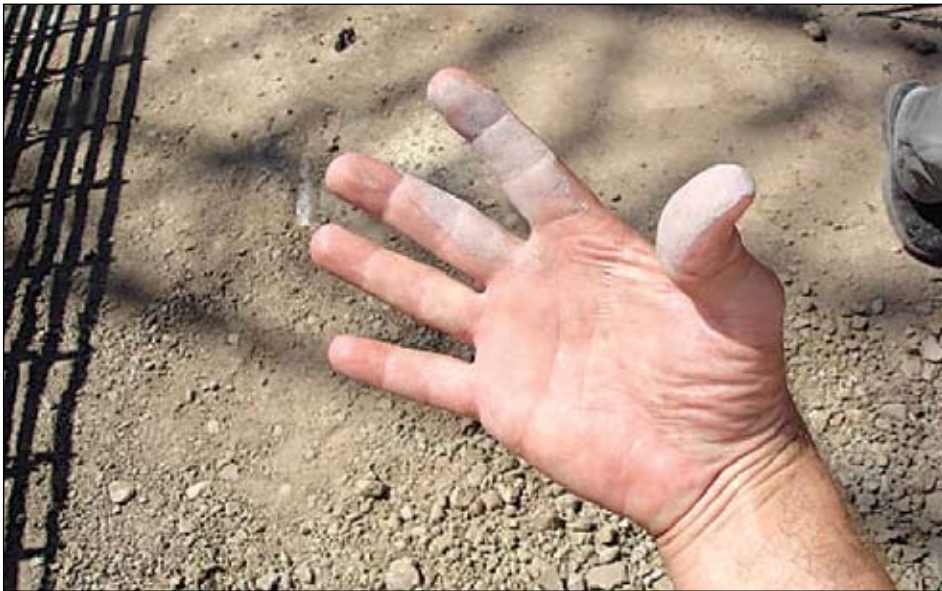
Figure 3 Smear contact from mudrock
