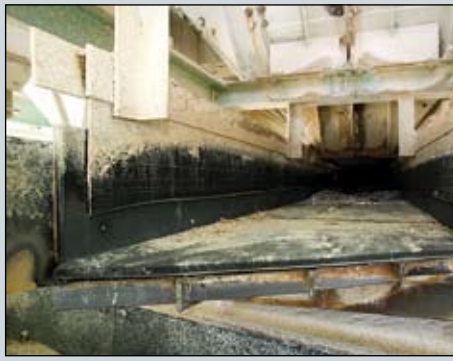
A view of the end of vibrating feeder VF01 in the secondary crusher screen plant showing polyurethane bottom and side liners, the side lining partially obscured by rubber curtains to prevent spilling. The picture was taken in mid-January 2006, 11 months after installation
