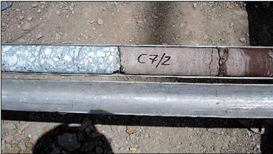
Figure 8 Pile contact on C7/2
