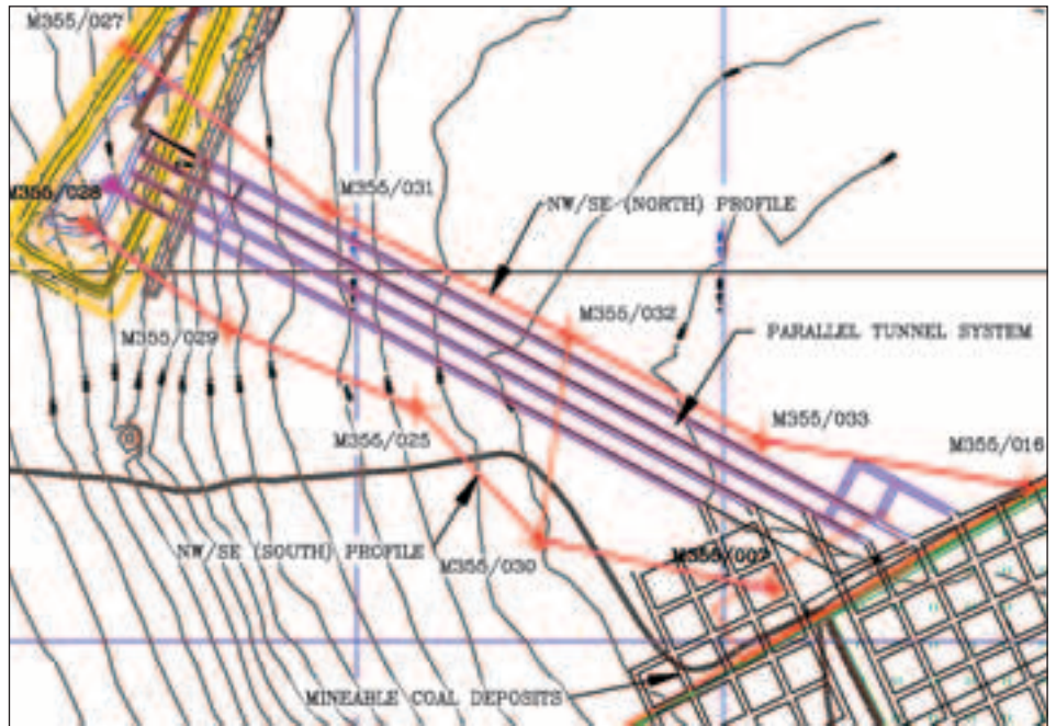
Layout of the four parallel access tunnels relative to the adit excavation and mineable coal deposits
