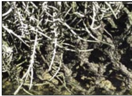
Encrusting of marine life on the woven mesh wire
