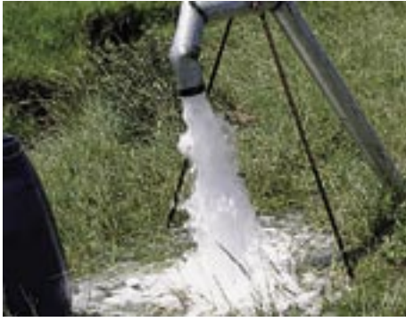
The photograph was taken during a test performed on the borehole. The yield of the final stage of the test was 45 ℓ per second, with the water level drawn down to 46 m below surface, after six hours of pumping
