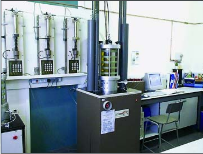
Figure 5 Hollow cylinder apparatus at the University of Southampton
