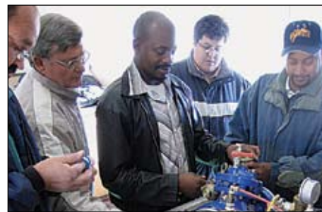
The test bench that was used to train delegates on setting of control valves under real flow conditions
