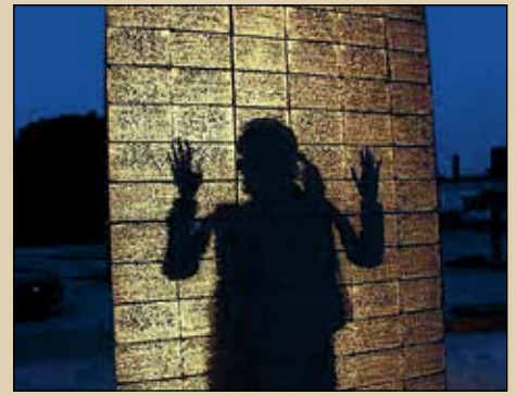
Translucent concrete offers a variety of interesting design possibilities
