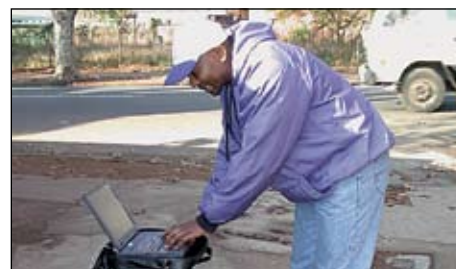
Trainer downloading a logger that is connected to a water meter
