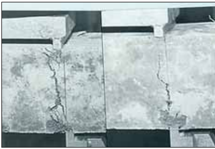
Figure 9 Two examples of failure lines in shear tests
