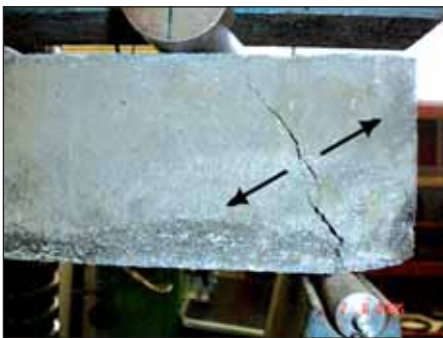
Figure 4 Shear crack at end of beam
