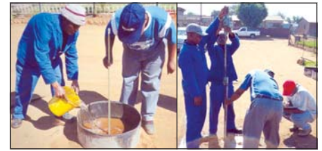
Figure 4 Soaked DCP test (Visser & Erasmus 2005)
